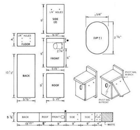
\* **Note**: If an oblong hole is not used, either drill a 1 1/2" hole or try a slot entrance. When given a choice, bluebirds build more nests in boxes with a front slot entrance, than in boxes with circular entrances. If a slot entrance is used the front will measure 5  $\frac{1}{2}$ " x 7  $\frac{1}{2}$ ". Leave the opening at the top.
