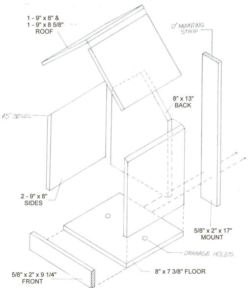
This can be made from one  $5/8'' \times 11'' \times 6'$  board  $(1 \times 12 \times 6')$  except for the mount
