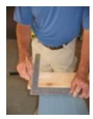
mark a straight line across your board. You can use a table saw if you have one, a circular saw or a hand saw. Make sure if you are using any type of power saw that you follow the manufacturer's instructions
