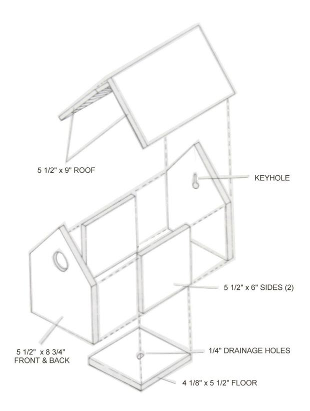
Take the front piece and measure up 6" from the bottom to center the 1 1/2" entrance hole. Measure to the same spot on the back piece to cut the keyhole for hanging the house. You can drill a 1/2" round hole for mounting if you wish.
